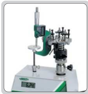
check the measuring force of micrometers
