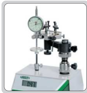
check the measuring force of dial indicators
