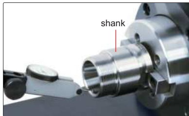
measure radial runout of shank
