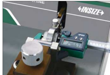
lapping measuring surfaces of outside micrometer
