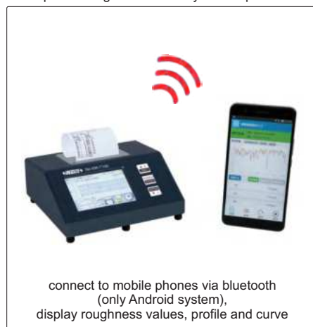
operate roughness tester by mobile phones
