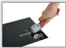
step 1: make grid cutting on surface
