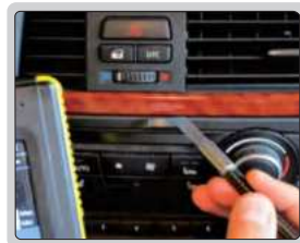
measuring gaps on the car dashboard
