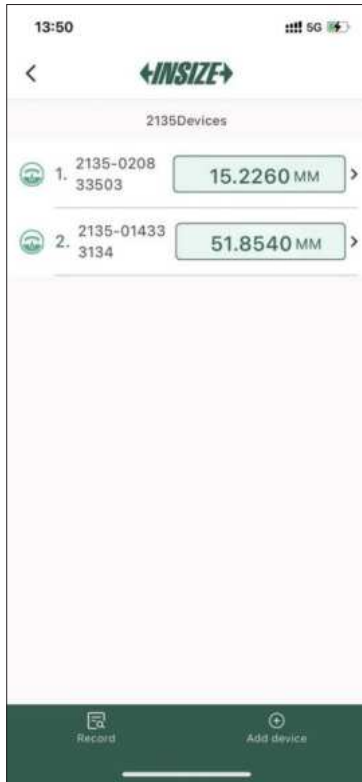
Real-time data from multiple digital indicators (up to 7pcs simultaneously connected)
