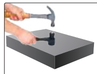
hammer impact to apply test force
