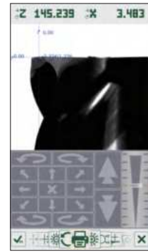
check cutting edge wear
