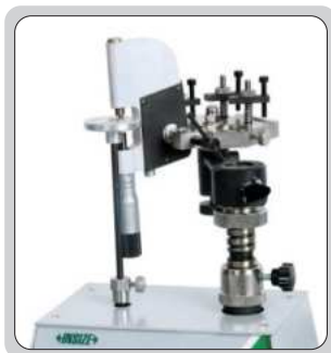
check the measuring force of indicating micrometers
